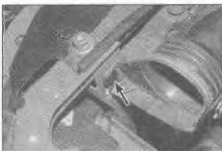
4.5 Push in the centre pin, then prise the complete plastic rivet (arrowed) from place, and remove the air inlet ducting
