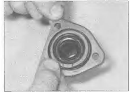
4.11 Fit a new O-ring/gasket (as applicable) to the guide sleeve
