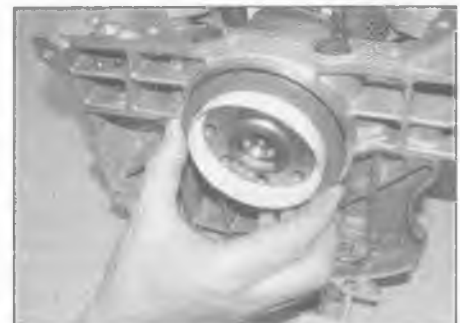
14.11 Locate the oil seal over the fitting sleeve and over the end of the crankshaft
