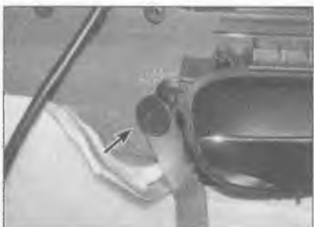
13.2 On front doors, prise out the interior door handle retaining clip (arrowed)
