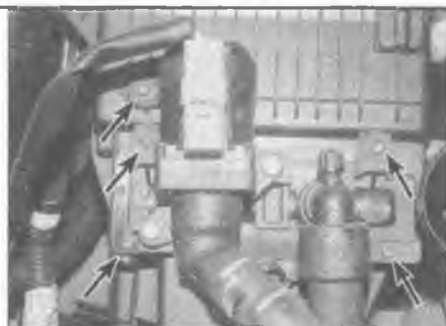
4.11 Undo the five screws (arrowed) securing the heater matrix into the air cleaner housing
