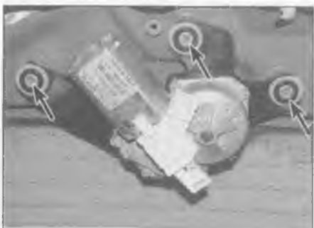
15.4 Drill out the three rivets (arrowed)
