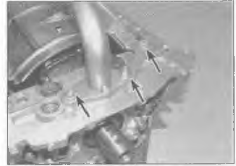
12.7a Oil pump pick-up tube retaining nuts and retaining bolt locations (arrowed)
