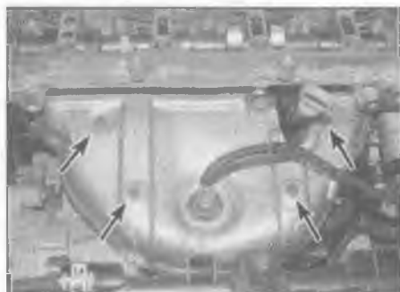
15.2a Undo the heat shield bolts (arrowed) . . .
