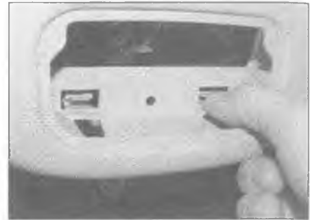
25.81 Release the two clips and pull the front of the console down
