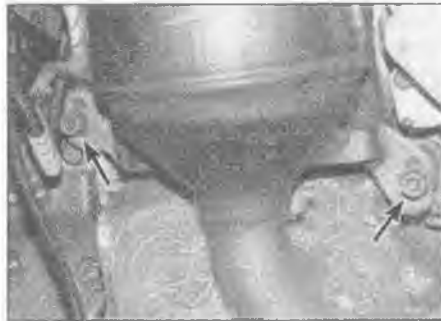
19.9 Catalytic converter mounting bolts (arrowed)
