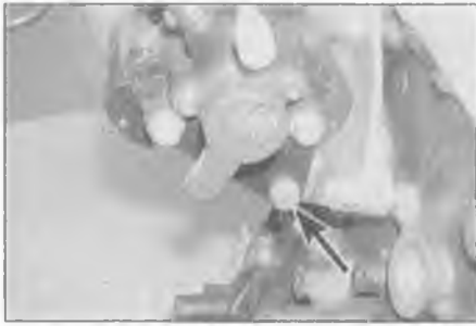
10.18 Undo the nut and bolt (arrowed) securing the fuel pump rear mounting to the mounting bracket
