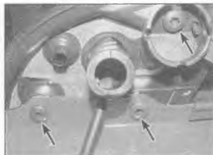
18.4 Undo the three screws (arrowed) and remove the mirror from the door frame
