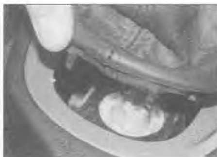
10.4a Unclip the gear lever gaiter . . .
