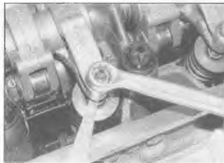
9.5 Check the valve clearances using feeler gauges
