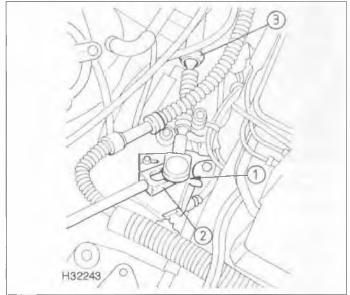
4.3 Prise off the selector cable balljoint (1) using a forked tool (2), then remove the cable from the bracket (3)
