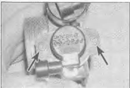
13.24 ... then undo the retaining screws (arrowed) and remove it from the throttle housing (1.4 litre engine)
