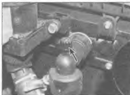
21.9b . . . and air cleaner heater matrix bleed screw (DW10ATED only)
