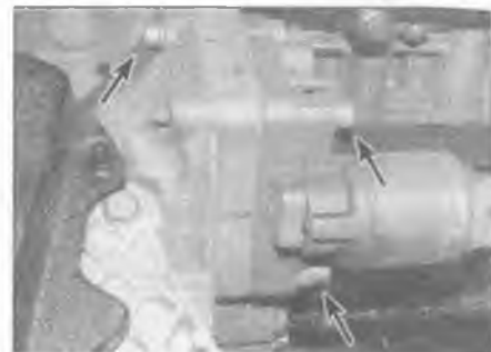
10.5 Starter motor mounting bolts (arrowed)
