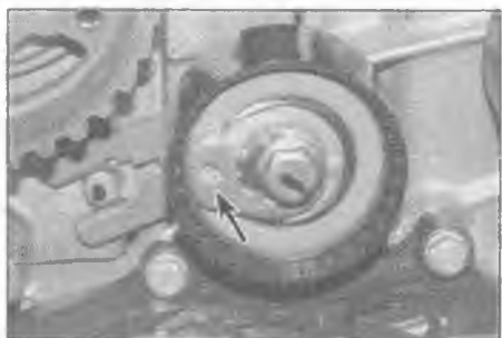
7.13 Insert an Allen key into the hole (arrowed), slacken the pulley bolt and allow the tensioner to rotate
