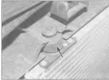
12.14a Ensure the condenser upper (arrowed) . . .
