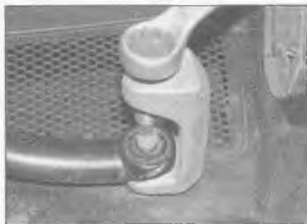
13.3 If the wiper arm is tight on the spindle, use a puller
