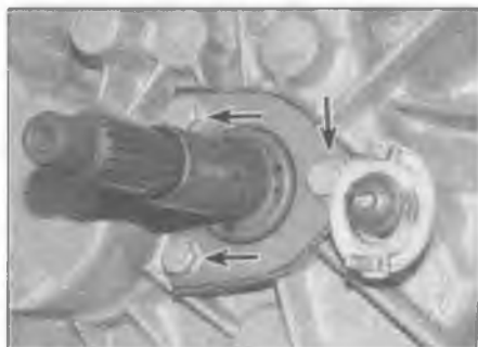
4.7 Undo the three bolts (arrowed) securing the guide sleeve
