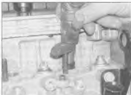
12.16 Withdraw the injectors, together with their clamps, from the cylinder head
