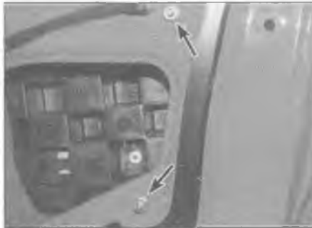
13.11 Undo the window rear guide channel retaining nuts (arrowed)
