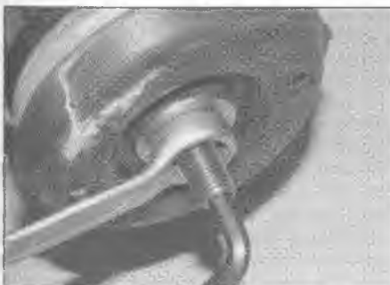
5.2 Slacken the top nut whilst retaining the rod with an Allen key
