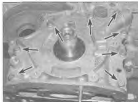
12.5 Undo the 8 bolts (arrowed) and remove the oil pump
