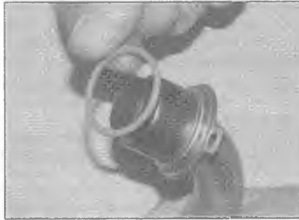
2.36c A new EGR pipe-to-manifold O-ring seal must be fitted
