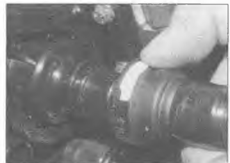
5.6a Press down the release button and disconnect the hose
