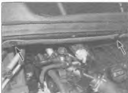
9.2a Prise up the centre pins, and lever out the plastic expanding rivets (arrowed) . . .
