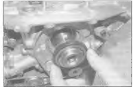
13.15 Slide the drive collar onto the crankshaft and engage it with the oil pump inner rotor
