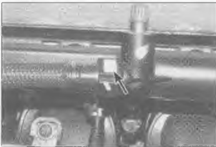
13.17 Depress the button (arrowed) and disconnect the fuel supply hose from the fuel rail
