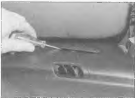
18.3 Carefully prise the tweeter cover from the fascia
