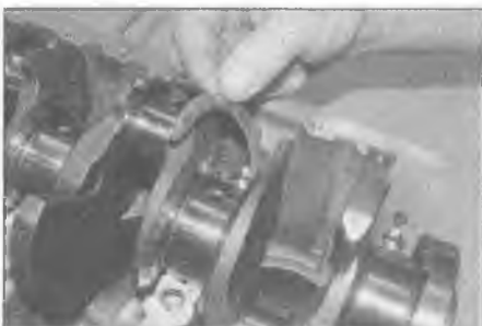
17.36 Insert the thrustwashers to either side of the No 2 main bearing upper location
