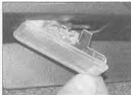
6.2 Prise the light unit from place (luggage compartment light)
