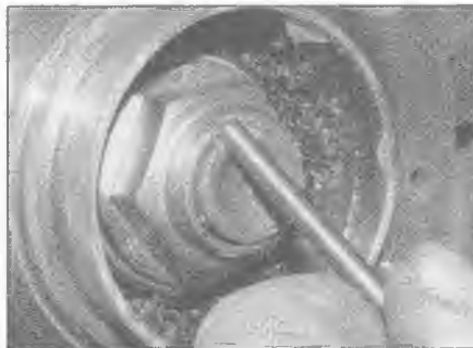
11.3 Unstake the retaining nut
