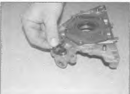
13.9 Locate a new O-ring over the oil pump outlet stub
