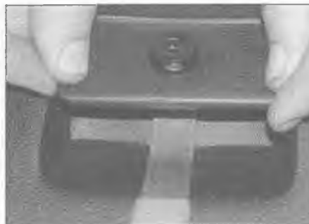
27.22a Insert a flat-bladed tool between the lock catch and the glovebox lid . . .
