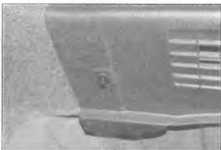
5.26 Prise up the centre pin, lever out the plastic rivets and remove the tailgate sill trim
