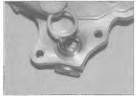
12.21a Fit a new oil seal . . .
