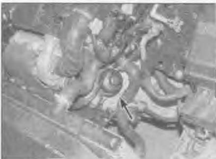
3.7 Engine oil filter cover (arrowed)
