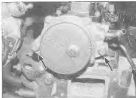
9.4 Undo the vacuum pump bolts (arrowed)
