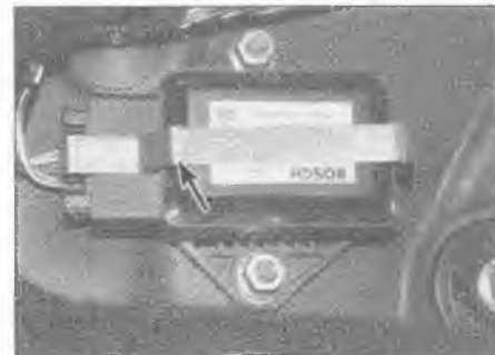
19.30 Release the clip (arrowed) and disconnect the Yaw rate sensor wiring plug
