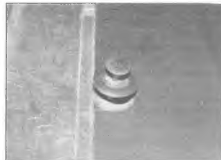
6.6a Prise up the centre pins, and lever out the expansion rivets
