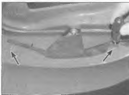
7.3 Remove the bolt and plastic rivet beneath the rear light aperture (arrowed)
