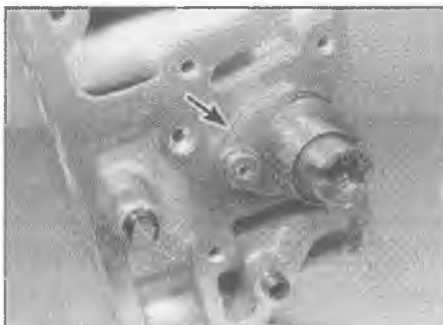
10.9 Undo the bolt and slide out the camshaft thrust fork (arrowed)
