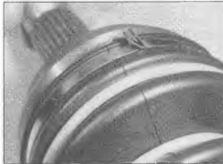
3.11i Fold the clip end underneath the buckle . . .
