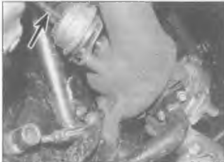
17.15 Turbocharger vacuum control pipe (arrowed)
