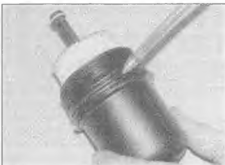
3.11b . . . and apply a little clean engine oil to the O-ring seal
