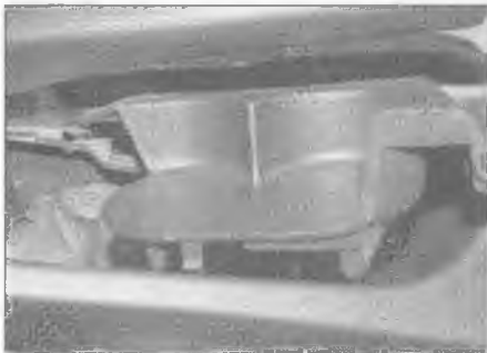
26.2 Pull up the storage tray/cup holder from in front of the handbrake lever
