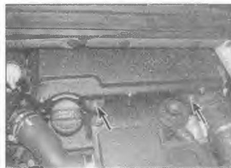
4.4a Undo the two air cleaner housing screws (arrowed)
