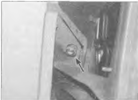
6.4 Undo the bumper-to-wing screws (arrowed)
