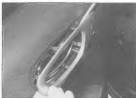
12.8 Carefully prise the handle surround trim from place (Estate/SW models)
