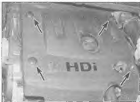
4.1 Rotate the four fasteners (arrowed) 90° anti-clockwise and pull up the plastic cover
