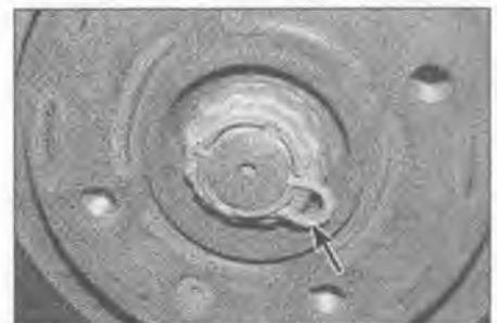
2.1 Prise out the R-clip (arrowed), remove the locking collar and slacken the driveshaft nut
