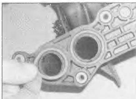
14.9a Ensure new manifold seals are fitted (1.4 litre engine) ...
