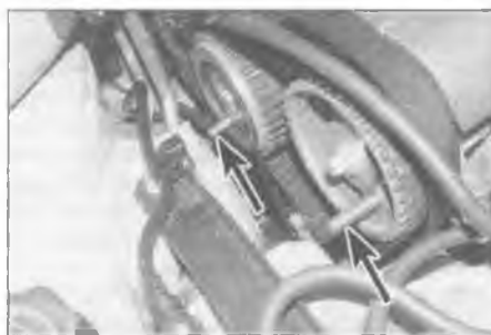
3.6 Camshaft sprocket locking tools (arrowed) inserted through the timing hole in each sprocket
