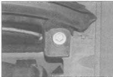
14.3c ... then undo the bolts (one at each end), and remove the plastic scuttle crossmember
