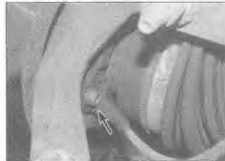
19.15 Undo the wheel speed sensor bolt (arrowed)
