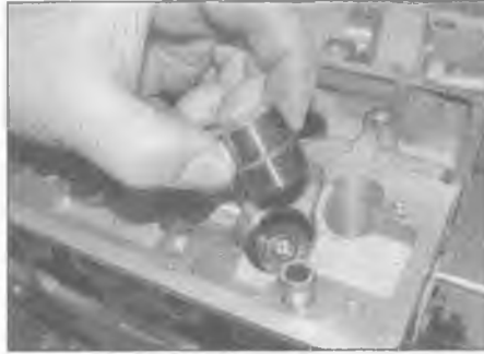
10.14b . . . then refit the tappets ensuring that each is refitted to its original bore
