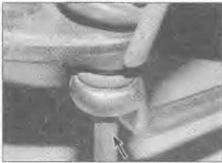
2.7 Use a Torx bit (arrowed) in the balljoint end to counterhold the nut
