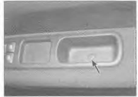
12.1a Undo the screw (arrowed) . . .
