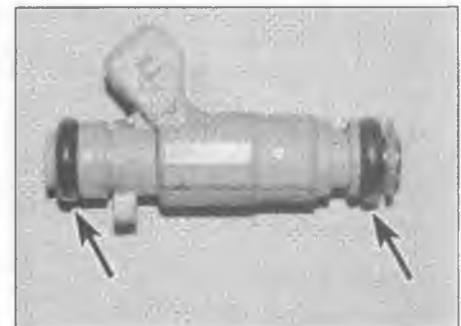
13.13 Renew all injector seals (arrowed) disturbed on removal
