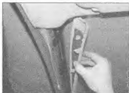
25.3 Unclip the trim from the A-pillar
