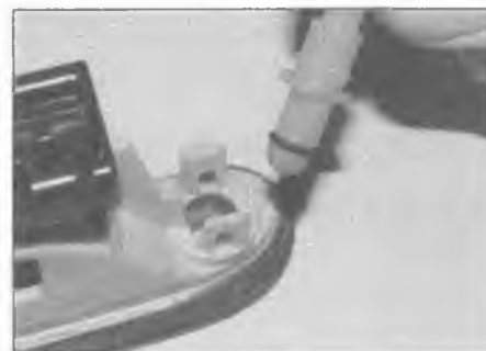
16.18 Release the clips and remove the washer jet
