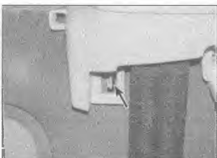
25.10 Release the clip (arrowed) and pull the trim from place
