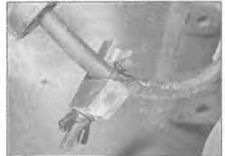
8.2 To minimise fluid loss, fit a brake hose clamp to the flexible hose
