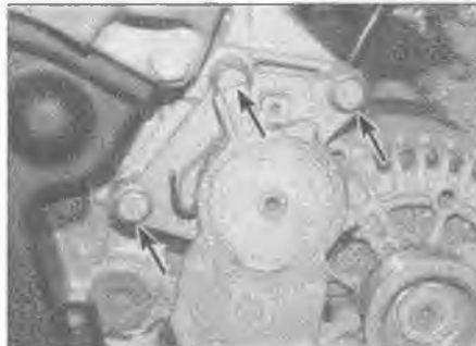
7.5 Undo the auxiliary drivebelt tensioner bolts (arrowed)
