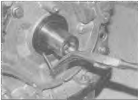
14.3 Drill a hole then use a self-tapping screw and pliers to extract the oil seal
