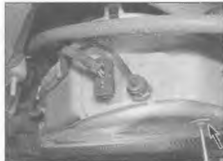
2.59 Additive reservoir heat shield retaining bolt (arrowed)
