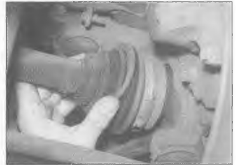
7.1 Check the driveshaft gaiter for damage
