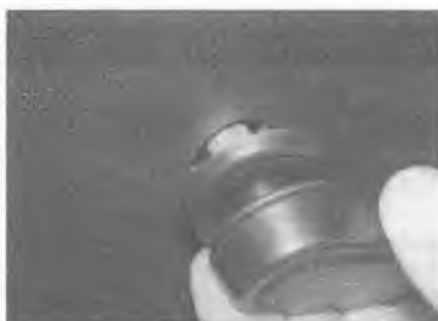
12.10 Pull the manual window winder handle from the spindle
