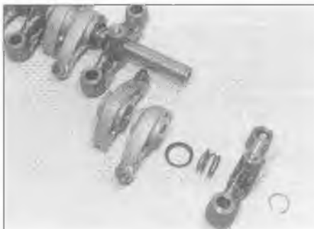
10.4 Remove the circlip and slide the components from the rocker shaft
