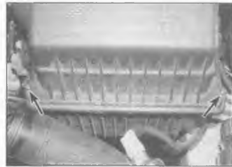
14.5a Undo the air filter cover screws (arrowed), lift off the cover . . .
