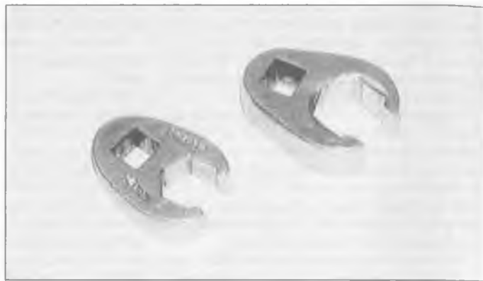
2.7 Two crow's-foot adaptors will be necessary for tightening the fuel pipe unions
