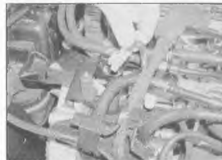
11.10b . . . and at the piston de-activator switch on top of the fuel pump
