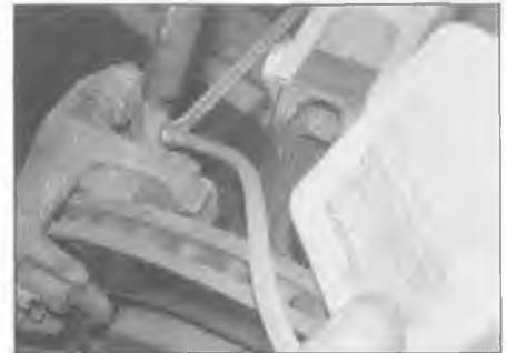
2.22 Connect the kit to the bleed screw
