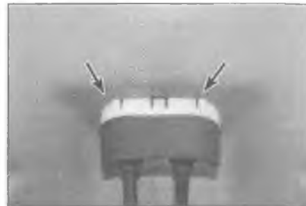
3.12 Depress the clips (arrowed) and release the cable sealing grommet from the floor
