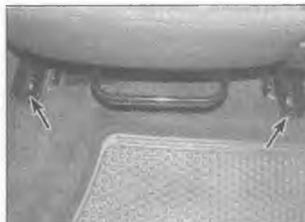
23.5 Undo the two bolts at the front of the seat rails (arrowed)
