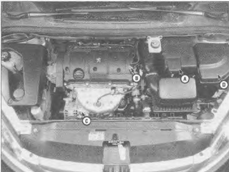
A Remove the plastic cover and check the condition and security of the battery connections.
