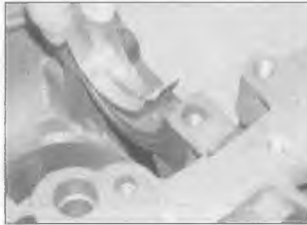
17.64a Ensure the grooved main bearing shells are fitted to the cylinder block . . .
