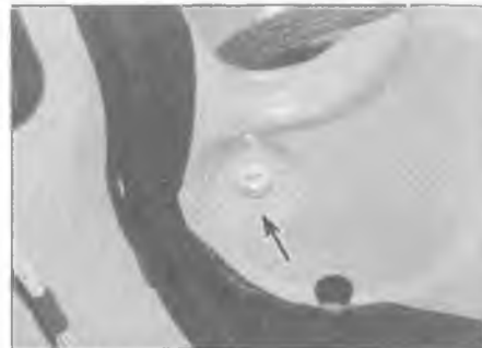
14.43 Drill out the front window guide rivet (arrowed)
