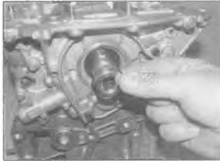
13.13 Position a new oil pump drive collar O-ring on the end of the crankshaft
