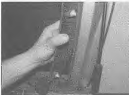
25.72 Unclip the two halves of the tailgate side trims
