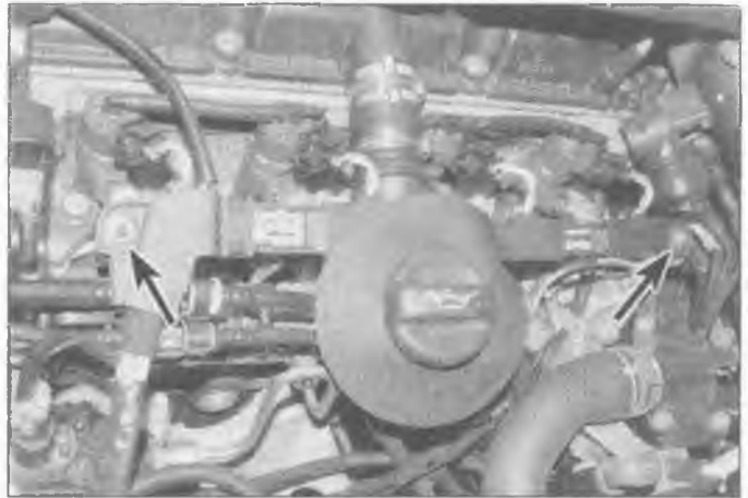
1.11b Undo the two nuts (arrowed) and move the wiring harness tray to one side
