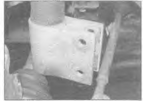
2.7b Rotate the base of the strut 90° towards the rear to minimise any chance of damaging the driveshaft gaiter
