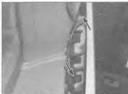
7.14 Two Torx screws secure the upper edge of the bumper (arrowed)
