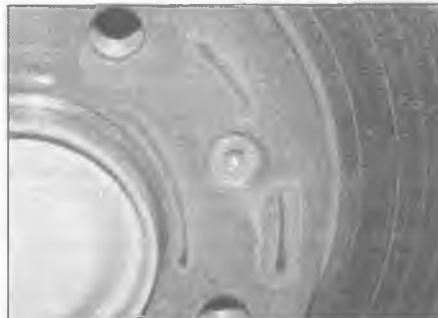
7.5 Undo the Torx screws and remove the disc
