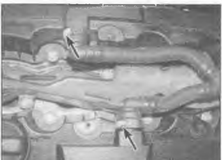
3.7 Depress the clips (arrowed) and disconnect the breather pipes
