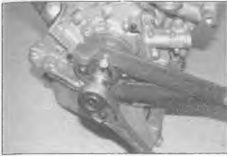
8.6a Hold the crankshaft sprocket end plate with the home-made tool while the retaining bolt is slackened
