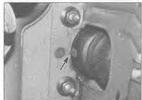
12.10 Release the servo retaining clips (left-hand one arrowed)
