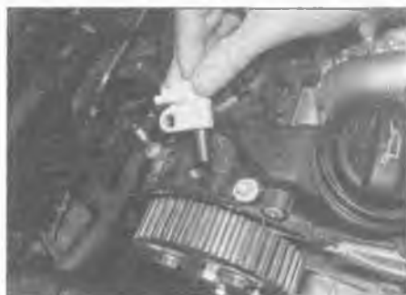
10.30 Remove the camshaft position sensor
