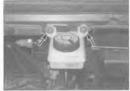
22.3 Undo the two screws securing the master cylinder upper reservoir (arrowed)
