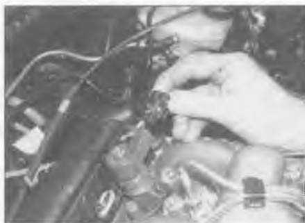
12.10 Disconnect the injector wiring
