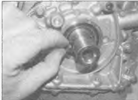
8.7 Remove the Woodruff key from the end of the crankshaft
