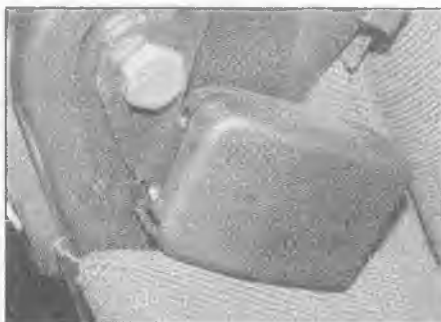
24.23 Undo the seat belt stalk bolt
