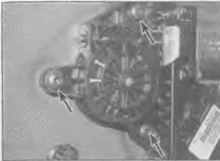
14.13 Undo the three Torx screws (arrowed) and remove the window motor
