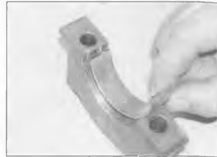
17.64b . . . and plain bearing shells to the bearing caps
