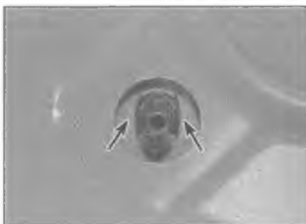
16.14 Squeeze together the clips (arrowed) and ease the jet from the bonnet
