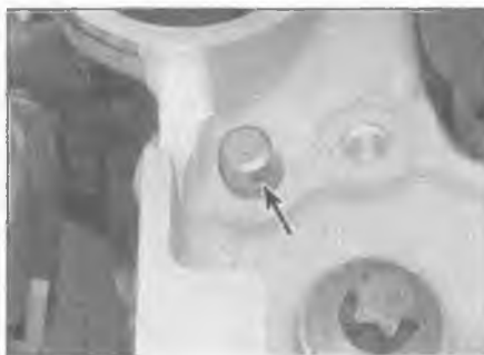
12.5c If it's loose, remove the locating dowel (arrowed)
