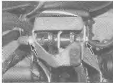
11.3 Slacken and remove the pivot bolt and nut (arrowed)
