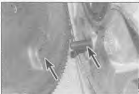
5.3 The locking pin/bolt (arrowed) must locate in the hole in the flywheel (arrowed) to prevent rotation
