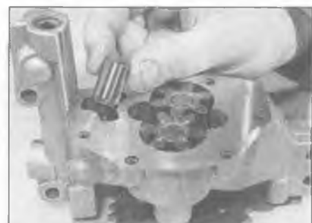
12.13c ... and relief valve piston, noting which way round it is fitted
