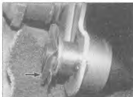
4.2 Remove the clip (arrowed) and slide out the bush
