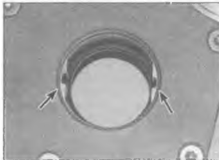
12.21b . . . align the pump gear flats (arrowed) . . .
