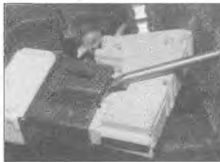
17.1 Lift the locking tab to disconnect the steering wheel lower wiring connector
