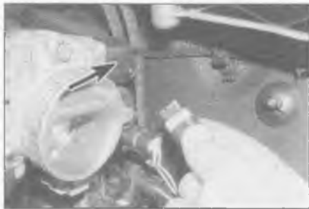
13.32 Disconnect the idle speed stepper motor wiring plug (arrowed) (1.4 litre engine)
