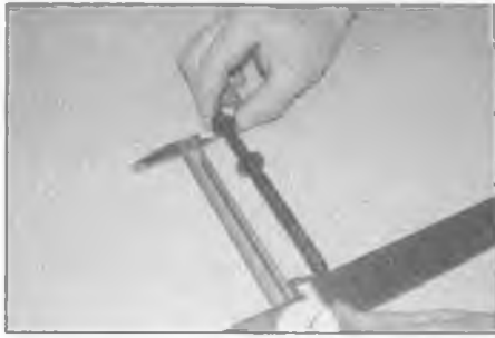
11.25 Measure the length of the cylinder head bolts from the underside of the head to the end of the bolt
