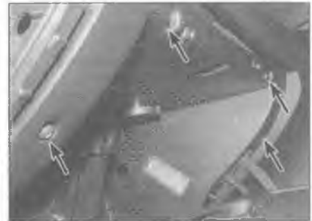
27.21a Open the glovebox and remove the 4 upper screws (arrowed) . . .
