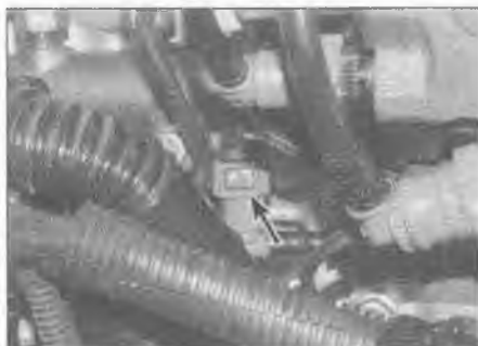
11.8 Depress the release button (arrowed) and disconnect the fuel return hose
