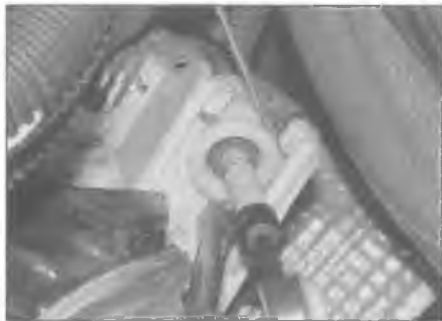
3.11a Depress the clip tabs and lever the cable outer upwards
