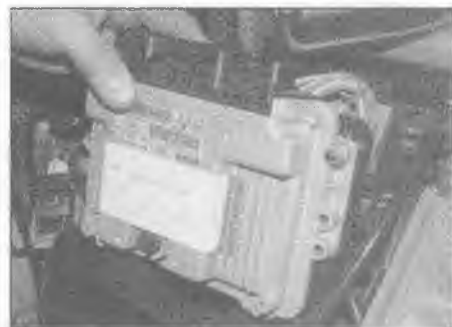
13.29 Lift the ECU up from the electrical box
