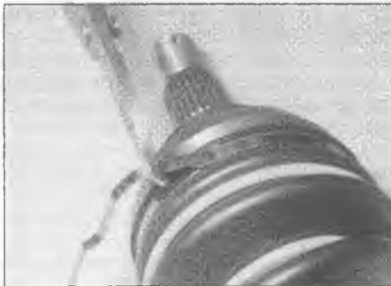
3.11h Bend the clip end back over the buckle, then cut off the excess
