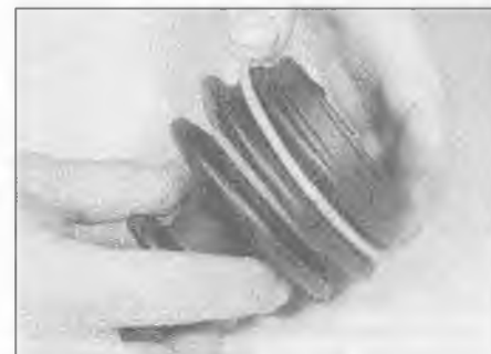
3.11a Fit the hard plastic rings to the outer CV joint gaiter . . .
