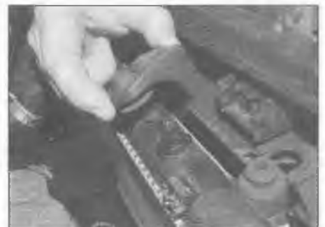
4.4b . . . and remove the radiator upper brackets
