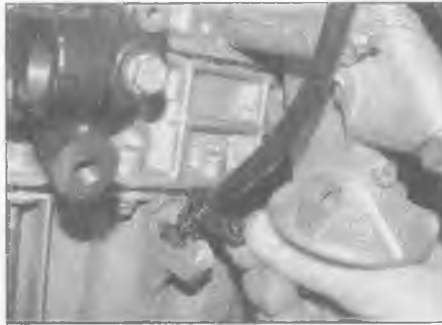
12.4 Undo the upper and lower retaining bolts and remove the dipstick guide tube
