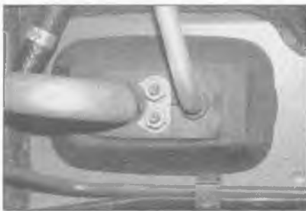
10.47 Undo the two nuts securing the air conditioning pipes to the engine compartment bulkhead
