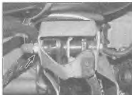
5.4 The clutch pedal bolt (arrowed) is also the pivot for the brake pedal
