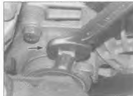
13.8 Use an open-ended spanner to rotate the tensioner arm clockwise, then lock it in place by inserting a 4 mm drill into the hole in the tensioner body (arrowed)
