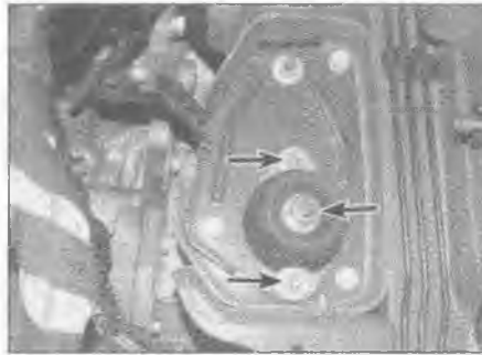
9.16a Undo the centre nut (arrowed), followed by the mounting retaining nuts (arrowed) . . .
