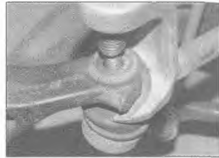
24.4b . . . then use a balljoint separator to release the tapered shank
