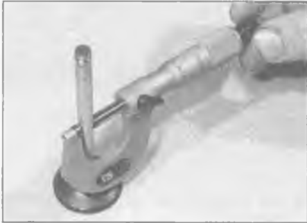
7.11 Measure the valve stem diameter with a micrometer
