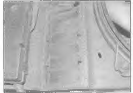
6.4a Release the retaining clips and remove the louvered panel . . .
