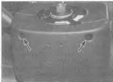
27.14a Two screws (arrowed) secure the steering column lower shroud
