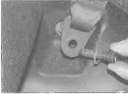
24.10 Undo the seat belt anchor bolt
