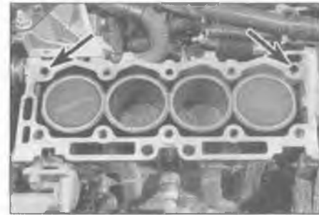
11.24 Ensure the locating dowels (arrowed) are in position then fit the new head gasket
