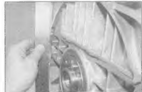
12.13 Use a straight-edge to ensure the rear faces of the cylinder block and sump are flush
