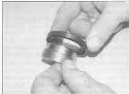
13.14b . . . and carefully fit the seal over the oil pump drive collar
