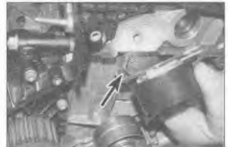
8.22 Ensure the slot (arrowed) on the tensioner pulley body engages with the web on the cylinder block when refitting
