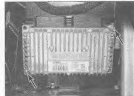
8.3 Undo the ECU mounting nuts (arrowed)
