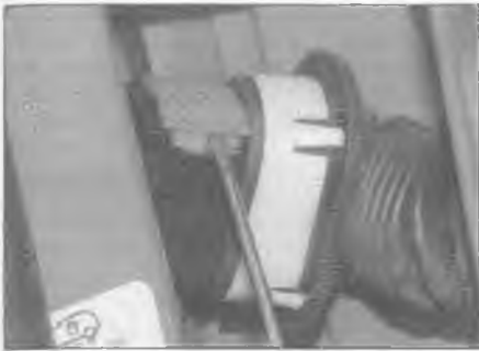
11.2 Lever up the locking catch and disconnect the wiring plug
