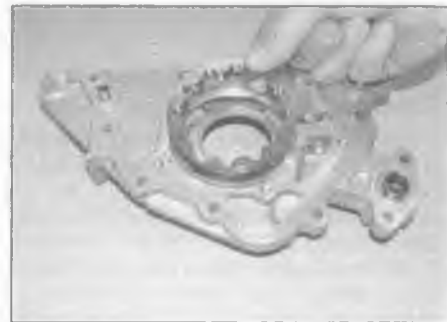
13.6c ... and outer rotor from the pump housing
