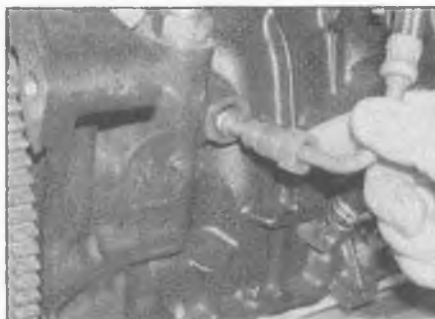
15.7 Unscrew the turbocharger oil feed pipe union nut
