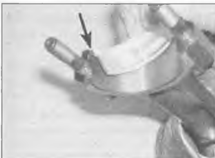
18.3 Ensure the bearing shell tab (arrowed) locates correctly in the cut-out
