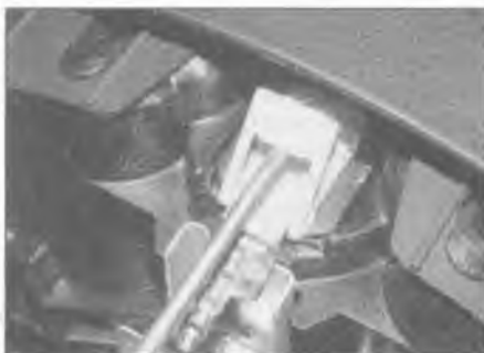
22.3b . . . by lifting the locking clip and sliding them from place
