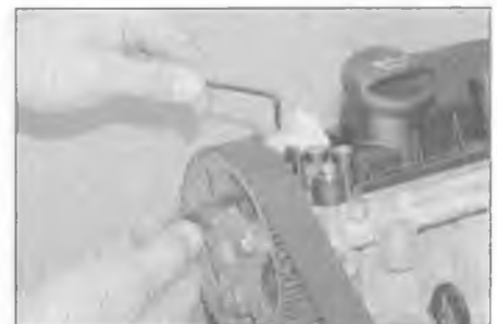
13.32 Insert feeler gauges bent 90° through the sprocket to measure the camshaft position sensor air gap
