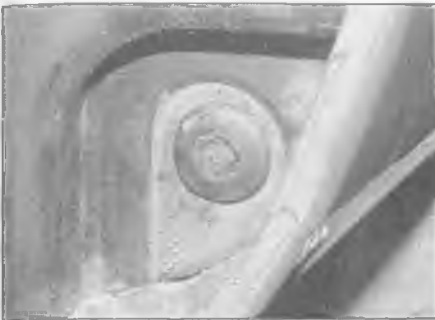
21.1a Push in the centre pins a little then prise out the plastic rivets
