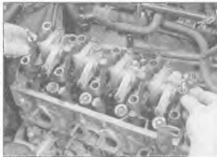
11.13 Lift off the rocker arm assembly
