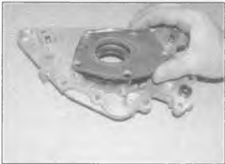
13.6a Undo the five screws and lift off the oil pump rear cover
