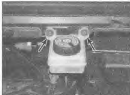
4.4 Undo the bolts (arrowed) and move the master cylinder upper reservoir to one side
