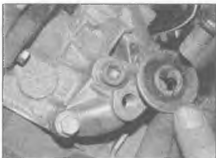
7.17 Remove the mounting stud and washer from the transmission casing
