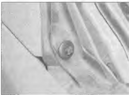
4.2a Push in the centre pin and prise out the complete rivet
