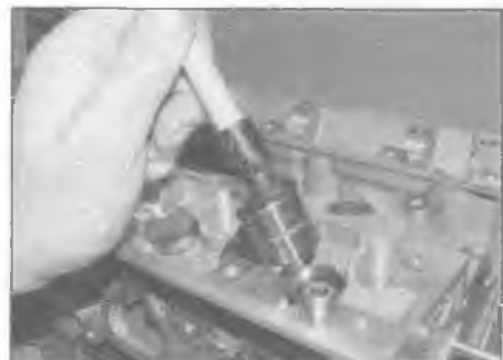
10.10 Use a rubber sucker to withdraw the hydraulic tappets
