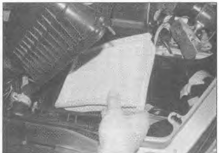
18.2 Note which way around the filter element is fitted
