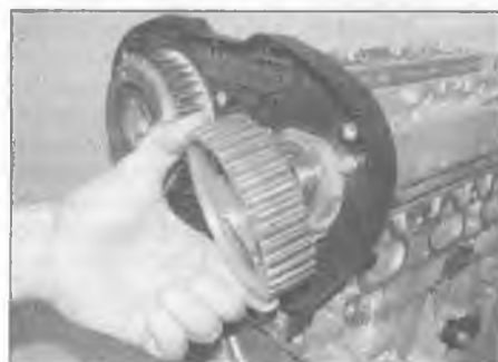
8.4b . . . and withdraw the sprocket from the end of the camshaft
