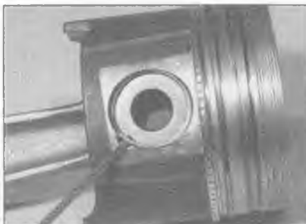
12.15a Prise out the circlip . . .
