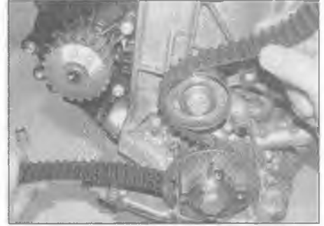
7.13a Retain the belt on the crankshaft sprocket and feed it over the idler pulley . . .
