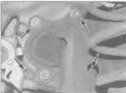
15.5 Undo the four bolts (arrowed) securing the stub axle to the lower arm
