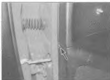
12.9a One screw (arrowed) is located at the front of the door trim ...
