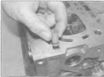
7.9b . . . and the camshaft oil supply non-return valve will be ejected from the underside of the cylinder head
