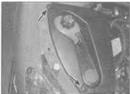
5.2 The cover over the reservoirs is retained by two plastic rivets (arrowed)
