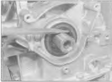
14.2 Use a screwdriver to lever out the crankshaft right-hand oil seal
