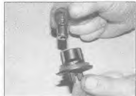
5.21b . . . then press in the bulb and rotate it anti-clockwise to remove it
