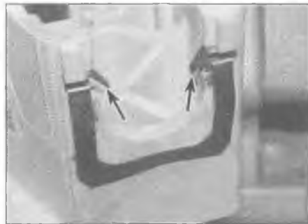
3.11b The cable retaining clip tabs (arrowed) – shown with the cable removed
