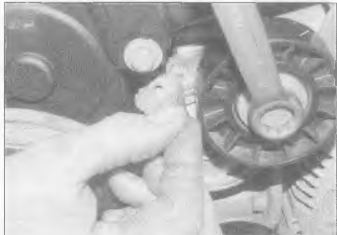
5.1a Insert a drill or pin to lock the auxiliary drivebelt tensioner in position (2.0 litre engines) . . .
