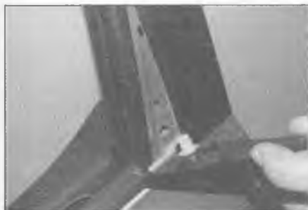
14.23 On Estate/SW models, prise the triangular shaped trim from the door exterior
