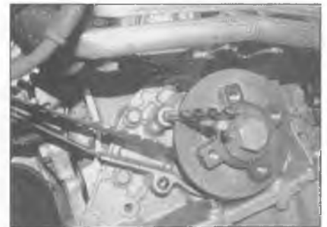
3.5 Insert an 8.0 mm drill bit or bolt through the hole in the crankshaft sprocket end plate, and into the corresponding hole in the oil pump housing
