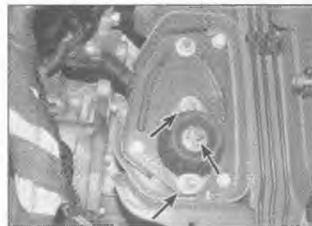
16.14 Undo the left-hand mounting centre nut and two retaining nuts (arrowed)
