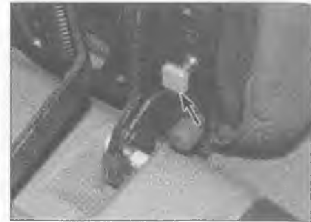
23.14 Release the clip (arrowed) and lift the seat from place
