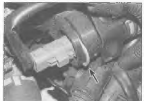
7.4 Prise out the clip (arrowed) and pull out the sensor
