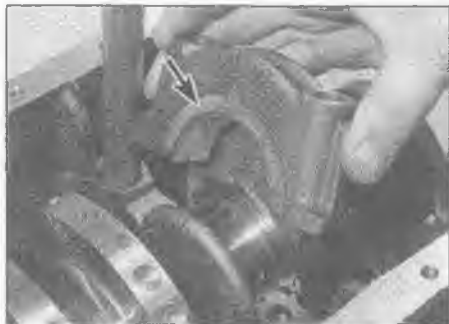
10.28 Note the thrustwashers (arrowed) fitted to the No 2 bearing cap
