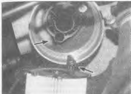
3.10b Ensure the filter locating peg (arrowed) locates into the corresponding hole in the housing (arrowed)
