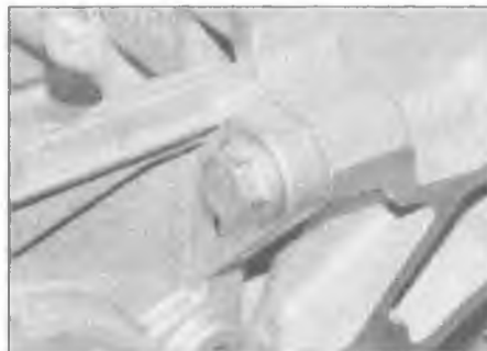
10.13b . . . and front support bracket upper bolt
