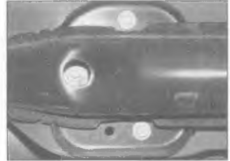
7.9 Undo the bumper bar bolts (left-hand side)
