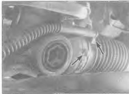
21.3 Rack gaiter breather pipe and inner clip (arrowed)
