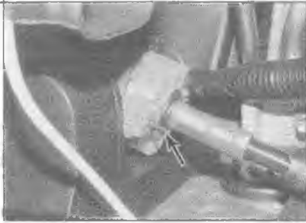
4.8b Pull out the pin (arrowed) a little, then slide up the outer cable fitting
