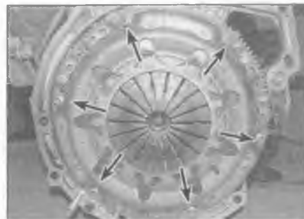
6.3 Undo the pressure plate bolts (arrowed)
