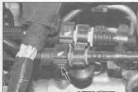
10.13 Press in the buttons (arrowed) and disconnect the fuel supply and return hose quick-release fitting at the connections
