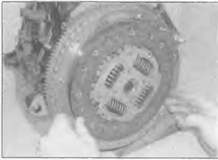
6.13 Fit the disc so the spring hub assembly faces away from the flywheel
