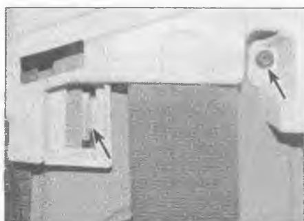
25.13 Undo the screw and clip at the lower edge of the trim (arrowed)
