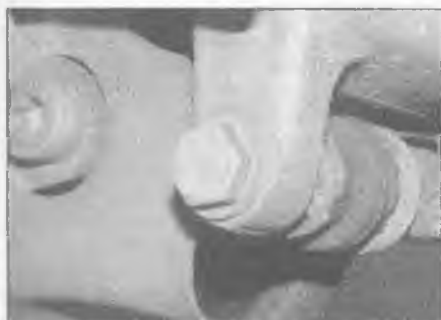
5.3 Remove the caliper lower guide pin bolt
