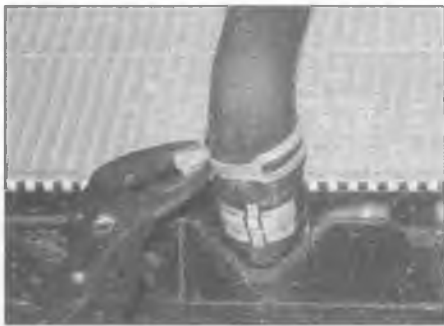
21.4 Squeeze together the tabs to release the hose retaining clip
