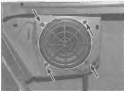
18.8 Rear speaker retaining screws (arrowed) (3-door Hatchback)
