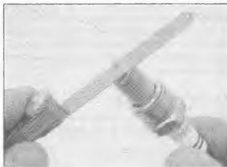
16.8 Measure the spark plug electrode gap with a feeler gauge
