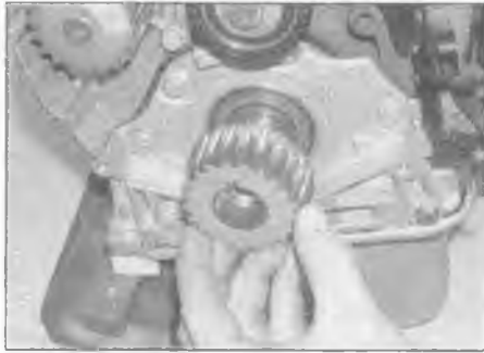
8.13a Slide the crankshaft sprocket off the end of the crankshaft . . .
