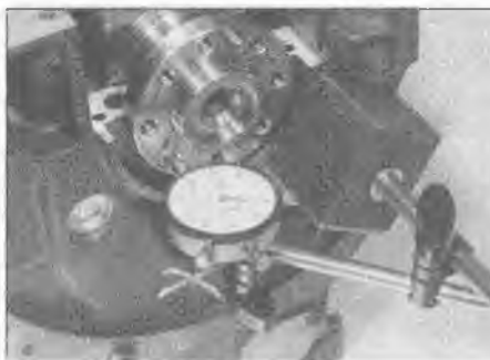
13.2 The crankshaft endfloat can be checked with a dial gauge ...
