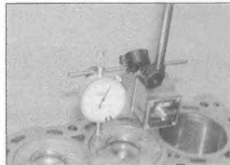
10.43 Measure the piston protrusion using a DTI gauge
