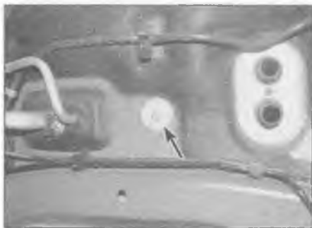
10.40 Heater/ventilation housing retaining bolt (arrowed)
