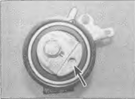
7.7 Using an Allen key in the hole (arrowed) on the tensioner pulley, rotate it clockwise to relieve tension from the belt
