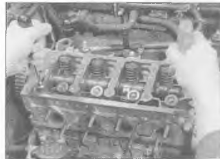
11.14 Use two stout screwdrivers to rock the cylinder head free from the block
