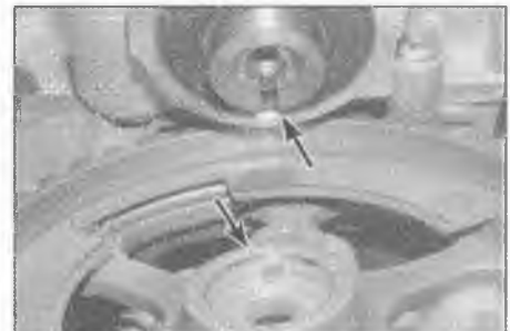
8.7 On 1.4 litre engines, align the sprocket lug with the notch in the end of the camshaft (arrowed)
