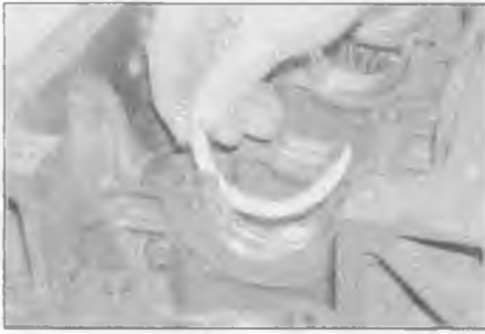
17.63 Fit the upper thrustwashers to the No 2 main bearing location with the oilway grooves facing outwards
