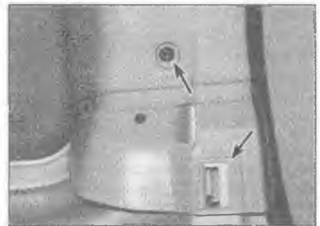
25.23 Undo the screw and release the clip (arrowed)
