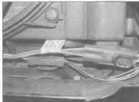
6.7 Disconnect the wiring plugs in the left-hand corner of the cooling fan panel
