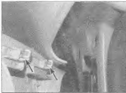
25.14 Release the clips (arrowed) at the upper edge of the trim
