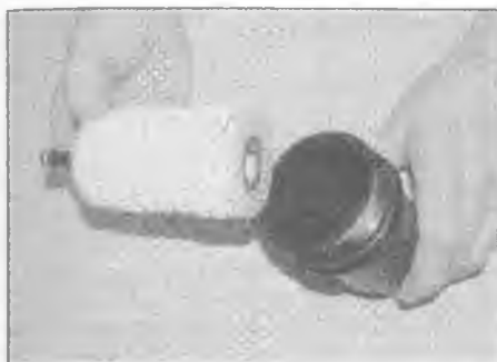
3.11a Fit the new element into the cover . . .
