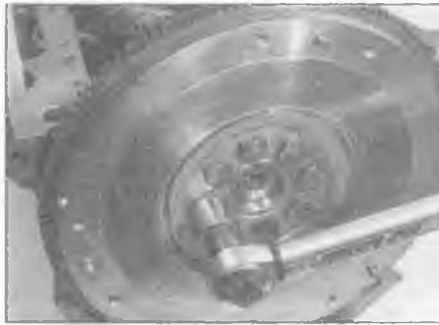
16.15 . . . then refit the flywheel and tighten the bolts to the specified torque
