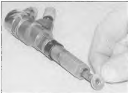
12.21b . . . and place a new copper washer on the injector nozzle
