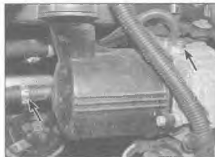
23.2 Disconnect the fluid pipes (arrowed) from the pump
