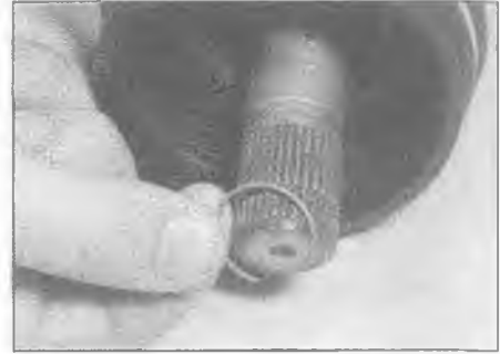
3.11d Fit the new circlip to its groove in the driveshaft splines . . .
