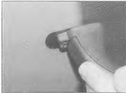
18.10 Slide the mirror up from the base
