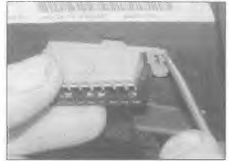
27.39 Depress the clip and push the diagnostic connector in
