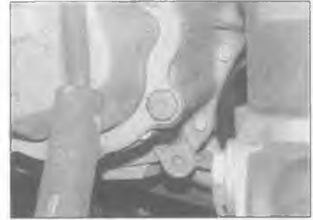
2.4b Oil filler/level plug (arrowed) (BE4/5 transmission)
