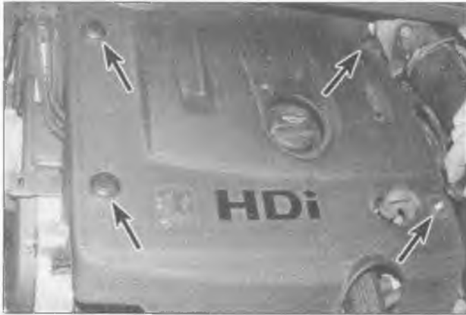
1.11a Rotate the four fasteners (arrowed) 90° anti-clockwise and pull the plastic cover from place
