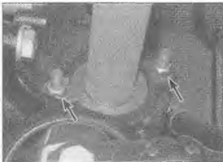
2.10a Slacken the two intermediate bearing retaining nuts (arrowed) . . .
