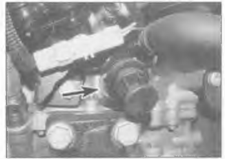
21.6 Prise out the retaining clip (arrowed) and pull out the drain plug
