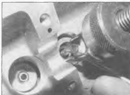
6.6b . . . then extract the collets and release the spring compressor
