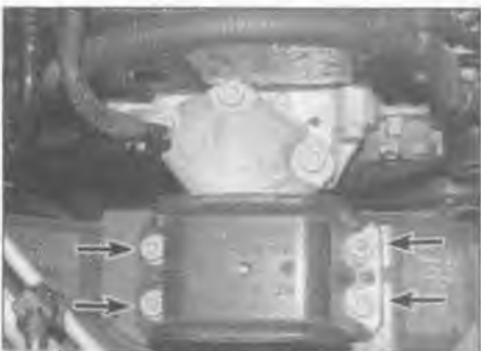
16.7 Undo the bolts (arrowed) and remove the engine mounting
