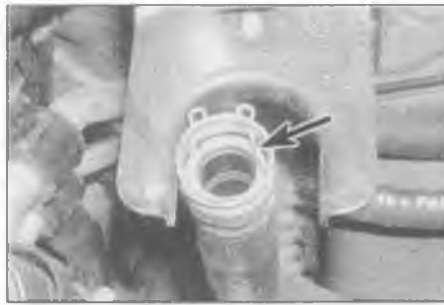
2.13 Ensure the sealing ring and circlip (arrowed) are correctly fitted to the hose union before reconnecting a connector
