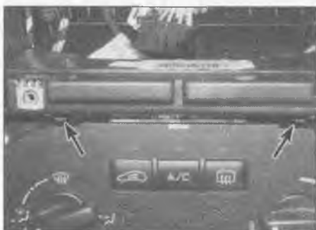
10.6b . . . and release the retaining clips (arrowed)
