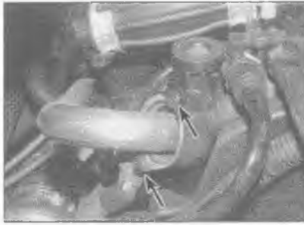
2.36a The EGR pipe is secured to the manifold by two screws (arrowed) . . .
