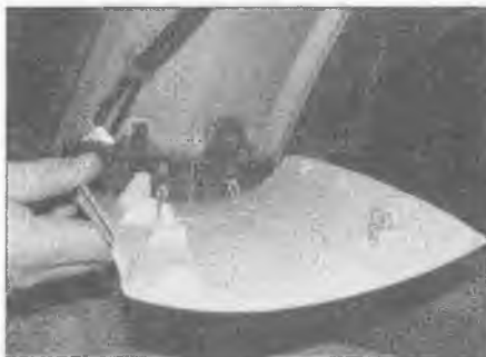
25.26 Pull the trim away from the pillar to release the clips
