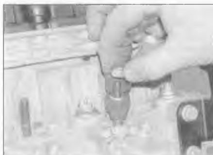
12.15a Unscrew the injector clamp retaining nut . . .
