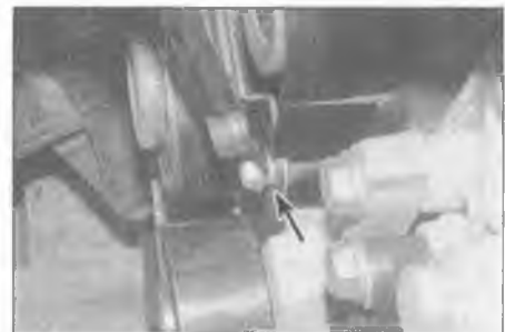
10.36 Ensure the lower edge of the inner timing belt cover engages correctly (arrowed)
