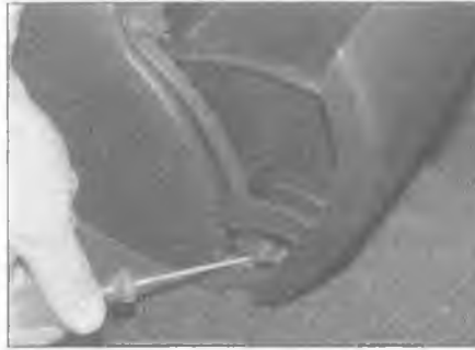
14.2 Gently prise out the lower edge and remove the ashtray
