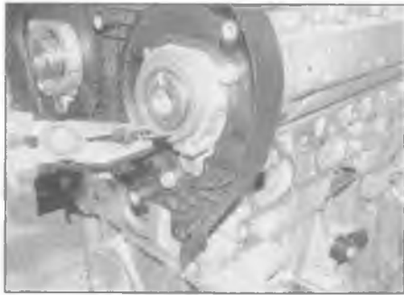
9.3 Use pliers and a self-tapping screw to extract the camshaft oil seal
