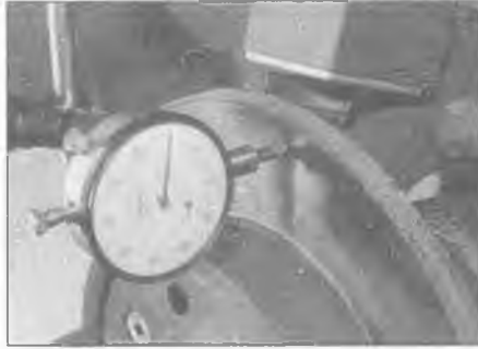
6.4 Check the disc run-out using a dial gauge
