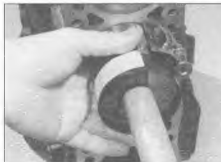
18.7 Tap the piston into the bore using a hammer handle
