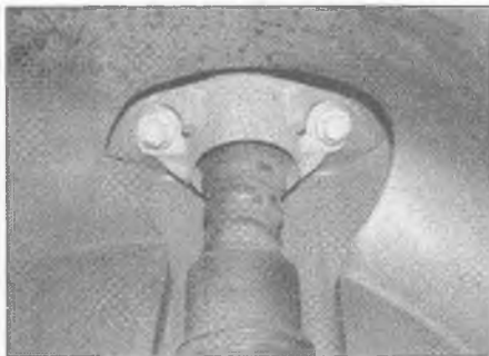
13.3 Undo the two shock absorber upper mounting bolts
