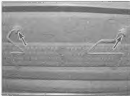
9.2 Undo the two nuts (arrowed) securing the fuel cooler
