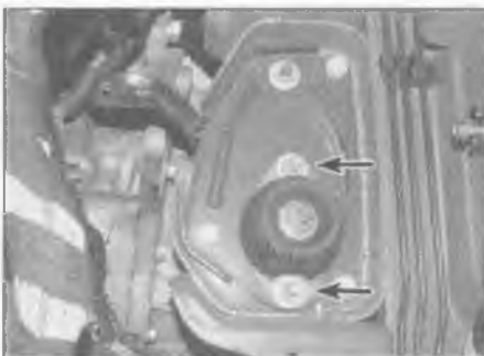
17.15a Undo the centre nut followed by the two mounting nuts (arrowed)
