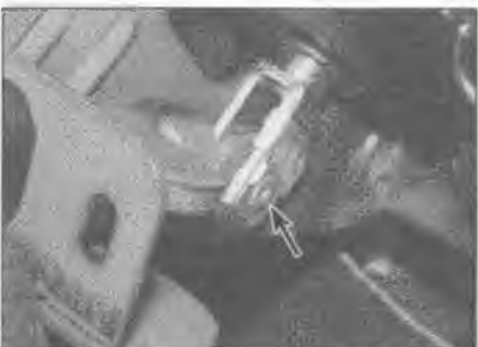
12.8 Rotate the clip (arrowed) then pull it from place
