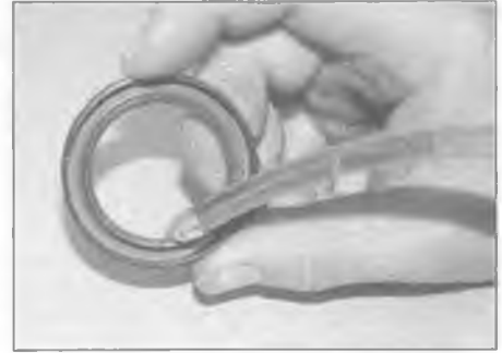
13.14a Lubricate the sealing lips of the new crankshaft right-hand oil seal . . .
