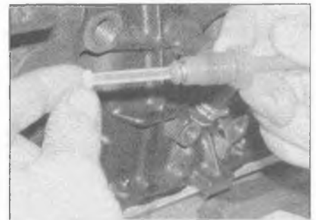
15.8 Withdraw the oil feed pipe and remove the filter
