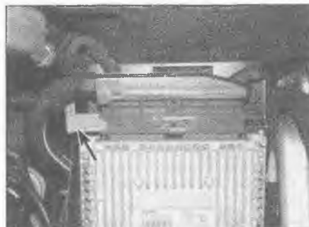
8.2 Slide out the locking catch (arrowed) and disconnect the ECU wiring plug
