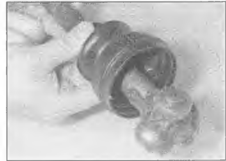
3.16b Slide the gaiter off the end of the driveshaft . . .
