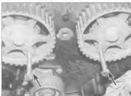
3.8 Use 10 mm diameter bolts/pins (arrowed) to lock the camshaft sprockets in position (1.6 litre engine)
