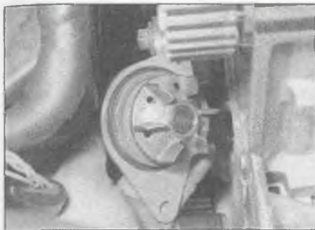
8.3a Remove the coolant pump . . .
