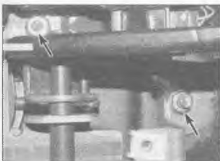
15.5 Undo the handbrake lever nuts (arrowed)
