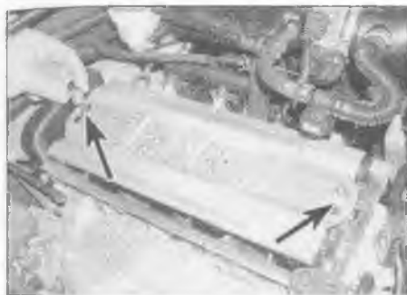
4.5a Remove the spacers (arrowed) from the studs . . .
