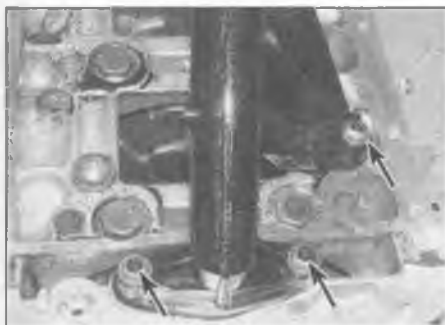
12.4 Undo the three Allen bolts (arrowed) and remove the oil pick-up tube
