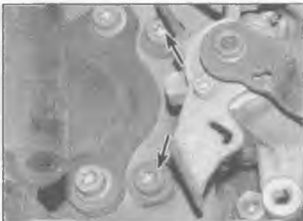
7.4 Slacken the two caliper mounting bracket Torx screws (arrowed)
