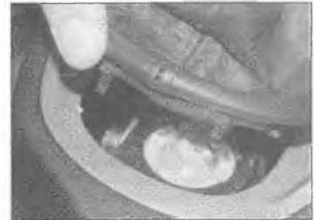
27.11a On manual transmission models, prise up the gear lever gaiter . . .
