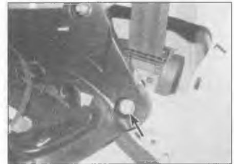
24.17b . . . and middle row seat belt inertia reel bolt (arrowed)
