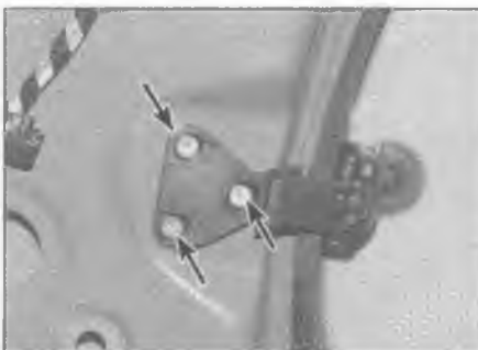
19.3 Drill out the three rivets (arrowed)
