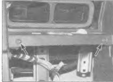
27.41 Undo the two screws (arrowed) in the audio unit aperture
