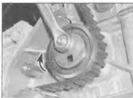
6.7 Slacken the nut then pivot the tensioner pulley clockwise to relieve the timing belt tension
