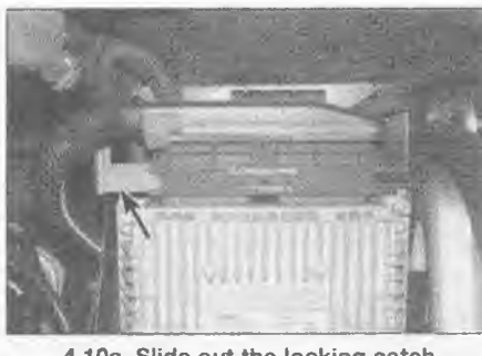
4.10a Slide out the locking catch (arrowed) and disconnect the automatic transmission ECU connector . . .
