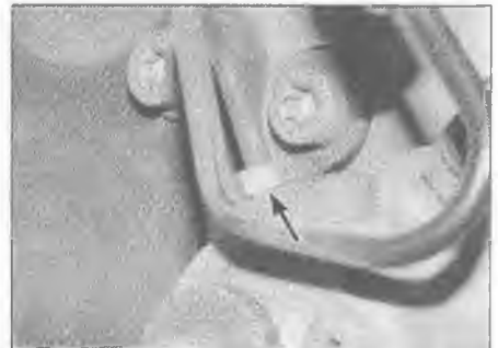
9.4 Unscrew the union nut (arrowed)
