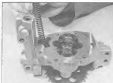
12.13b ... then lift off the cover and remove the spring ...
