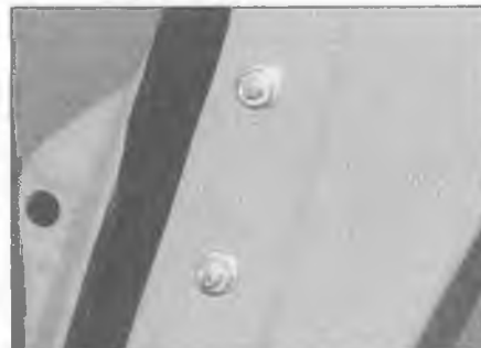
14.26 Undo the two nuts securing the window guide channel
