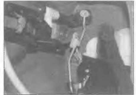
13.12 Unclip the link rod from the handle to the lock
