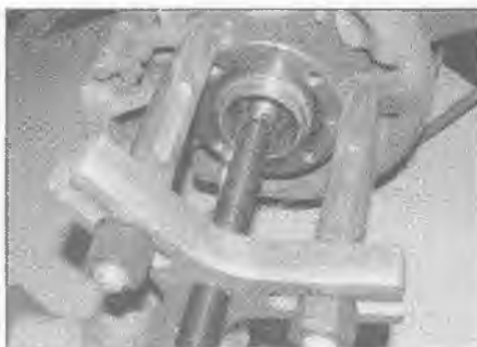
11.5 Use a puller to remove the hub
