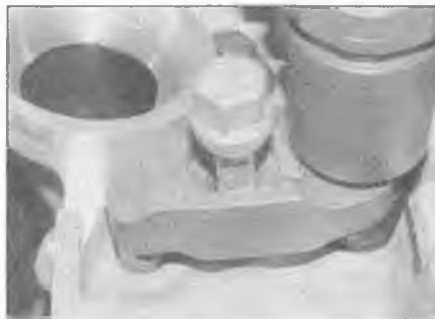
12.5a Undo the injector clamp bolt ...
