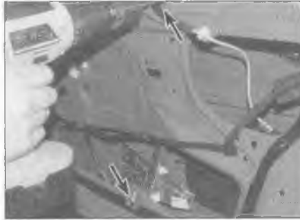
14.14 Drill out the two rivets (arrowed) . . .
