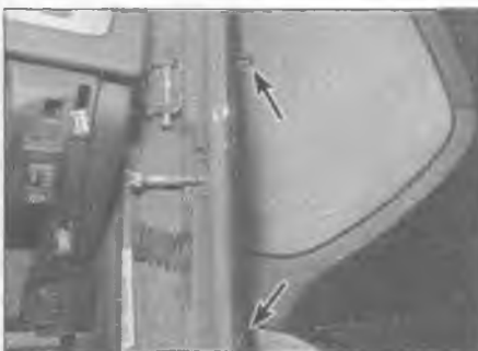
12.4a Undo the two screws (arrowed) at the front edge of the door trim . . .
