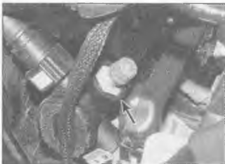
7.2 Fuel pressure relief valve (arrowed)
