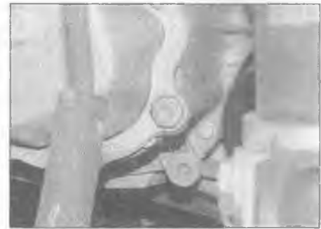
19.3b Oil level/filler plug (BE4 transmission)
