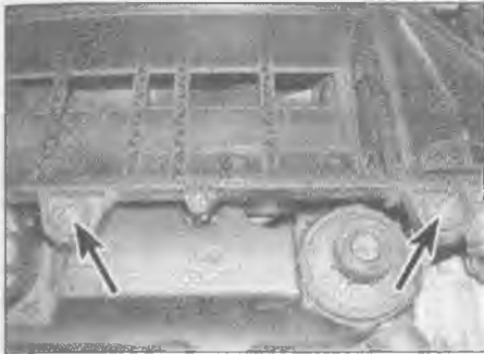
4.13 Undo the two bolts (arrowed) and pull the air filter housing up from its place
