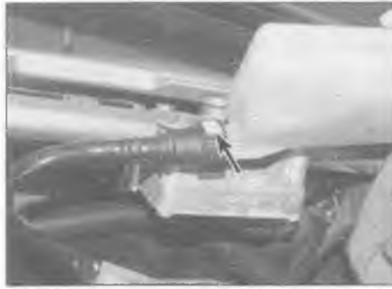
10.3b . . . then depress the button (arrowed) and disconnect the pipe
