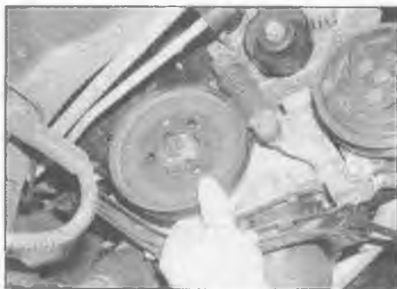
5.7b . . . and remove the crankshaft pulley
