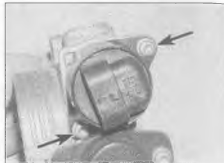
13.33 Undo the retaining screw(s) and remove the motor from the housing
