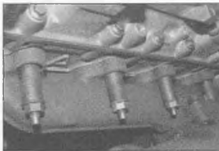
15.2a Undo the exhaust manifold nuts, recover the spacers, and remove the manifold
