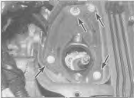
17.15b Undo the nut/bolts (arrowed) and remove the mounting support bracket
