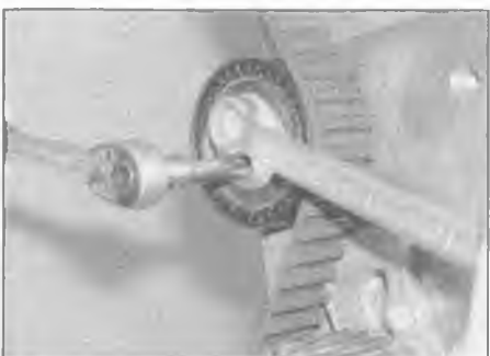
7.41a Pivot the tensioner pulley anti-clockwise, then tighten the retaining bolt . . .
