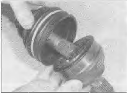
3.11e . . . then locate the joint outer member on the splines, and slide it into position over the circlip. Ensure that the joint is securely retained by the circlip
