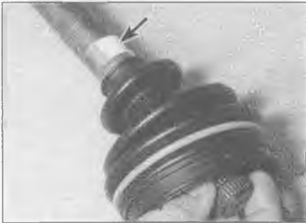
3.11b . . . then slide on the new plastic bush (arrowed – where fitted), and seat it in its recess in the shaft. Slide the gaiter onto the shaft . . .
