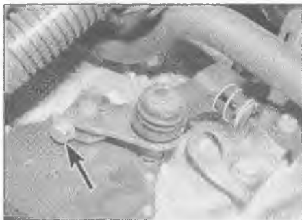
6.12 Unscrew the nut and clamp bolt (arrowed) and free the selector lever from the transmission shaft
