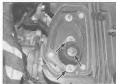
16.15a Slacken the centre nut (arrowed) then undo the mounting retaining nuts (arrowed)
