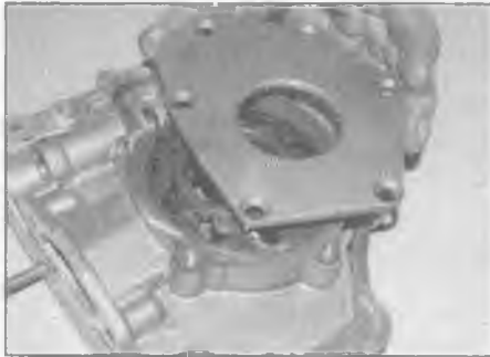
12.8 Undo the Torx screws and remove the pump cover
