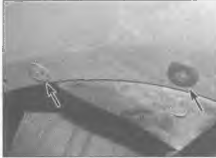
7.5 Push in the centre pins and prise out the plastic rivets (arrowed)
