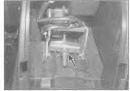
14.4 Equaliser plate adjustment nut (arrowed)
