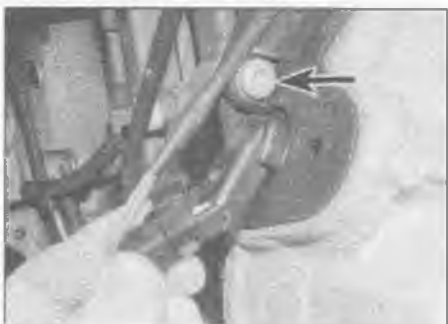
13.41a Disconnect the wiring plug then undo the retaining screw (arrowed) . . .
