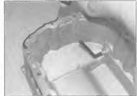
12.11 Apply a thin bead of RTV sealant to the sump mating surface
