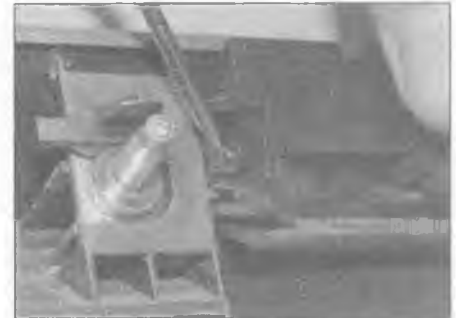
16.12 Release the clips and slide the handle out
