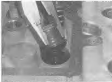
6.6f Use a pair of pliers to remove the valve stem oil seal. On 1.4 litre diesel and 2.0 litre petrol models the spring seat is integral with the seal
