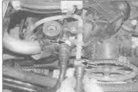
4.17 Depress the locking buttons (arrowed) and disconnect the fuel feed and return hoses
