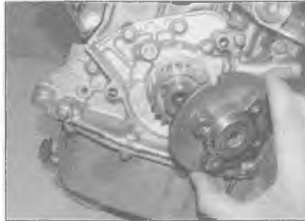
8.6b Withdraw the crankshaft sprocket end plate . . .
