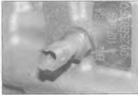
15.3a On 1.4 litre engines, the oil pressure switch is on the front face of the cylinder block
