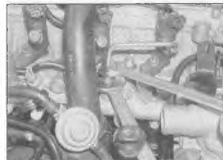
11.16a Using two spanners, unscrew the fuel pipe unions at the accumulator rail . . .
