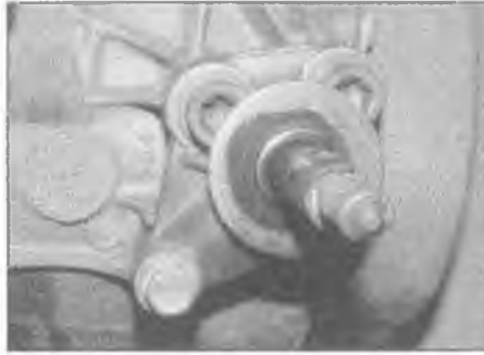
16.16 Unscrew the mounting stud from the mounting
