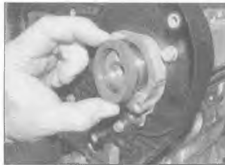
9.5 Locate the new seal in position with the seal lips facing inwards
