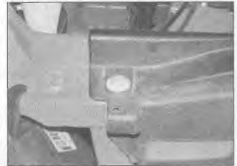
6.8a Undo the screw on the right . . .
