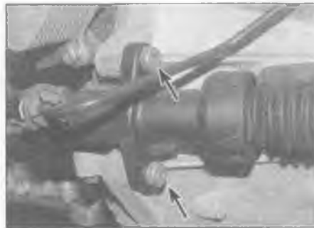
4.6 Undo the two bolts (arrowed) and remove the clutch slave cylinder
