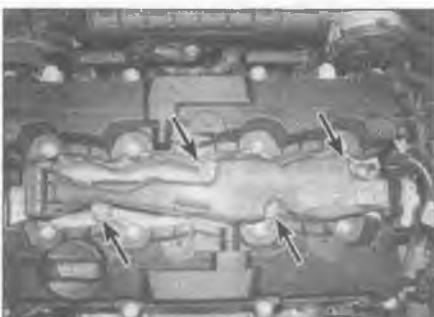
3.8 Undo the four coil pack retaining screws (arrowed)
