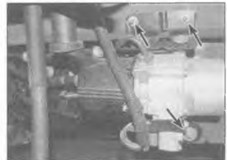
23.4 Undo the upper and lower pump mounting bolt/nuts
