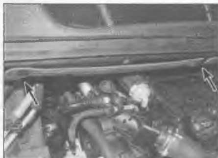
9.2a Prise up the centre pins, then lever out the complete plastic rivets (arrowed) . . .
