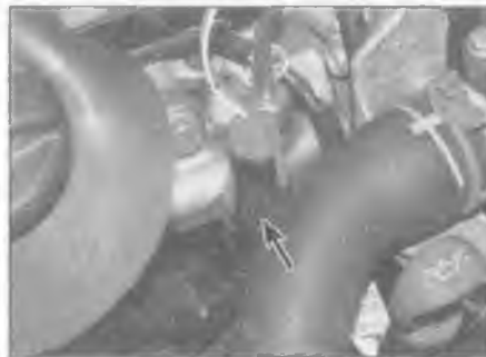
13.42 Fuel temperature sensor (arrowed) (2.0 litre engine)
