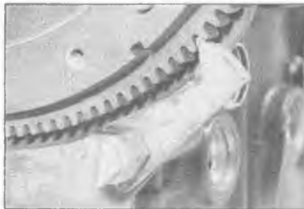
5.2 Use a fabricated tool similar to this to lock the flywheel ring gear and prevent crankshaft rotation
