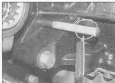
3.8 Rod (arrowed) inserted through the cylinder block into the flywheel timing hole (2.0 litre engine)
