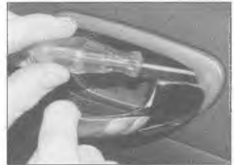
12.3 Insert a small screwdriver into the hole to release the retaining clip
