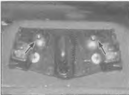
16.6 Undo the two bolts and remove the lock striker (arrowed)
