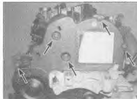
6.3 Undo the 5 screws (arrowed) and remove the upper timing belt cover
