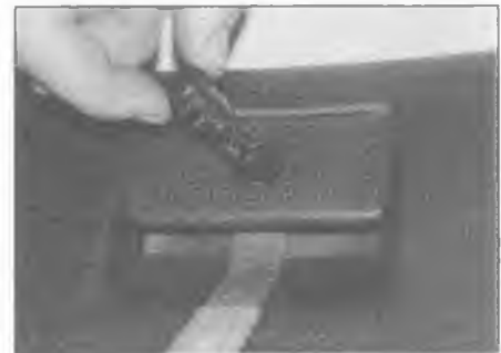
27.22b . . . then press the catch down to release the cylinder
