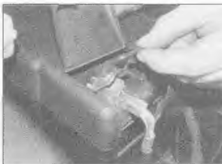
4.3a Lift up the quick-release lever and disconnect the positive lead . . .
