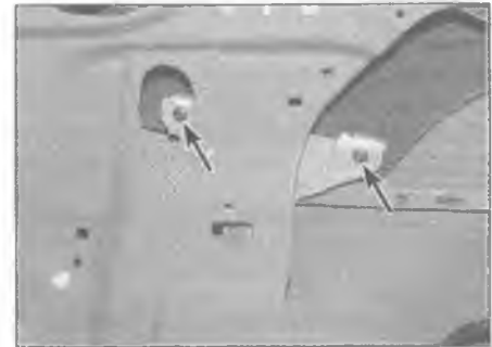
14.22 Undo the two window clamp screws (arrowed)
