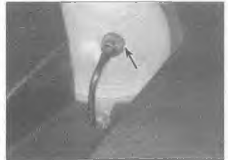
3.3a Slide up the retaining clip (arrowed) and pull out the hose
