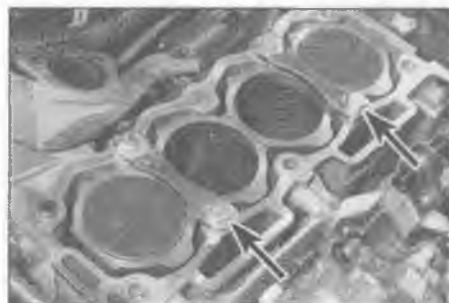
11.15 On 1.4 litre engines, clamp the cylinder liners in position before rotating the crankshaft (clamps arrowed!)
