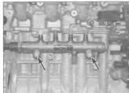
11.9 Remove the accumulator rail mounting bolts (arrowed)
