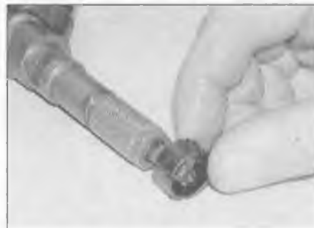
12.21a Locate a new upper seal on the body of each injector . . .
